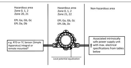
\*The temperature sensor assembly is shown for illustration purpose only. The remote mount or direct mount sensor, or its assembly with T142 is not covered by this certificate.
