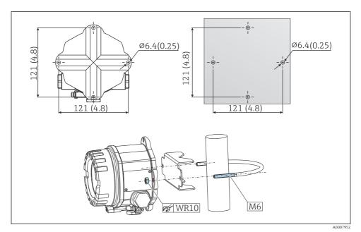
Mounting of the field transmitter via direct wall mounting or with a 2" pipe mounting bracket (316L, available as an accessory). Dimensions in mm (in)
