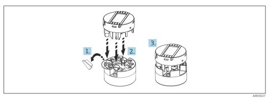
■ 16 Attach the display to the transmitter
