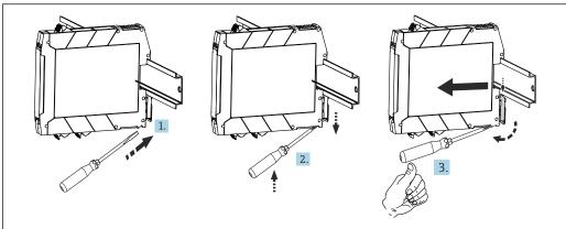
■ 8 Dismantling the DIN rail transmitter
