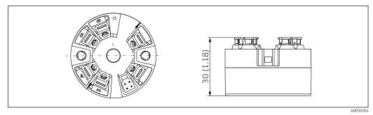
20 Version with push-in terminals. Dimensions are identical to the version with screw terminals, apart from housing height.
