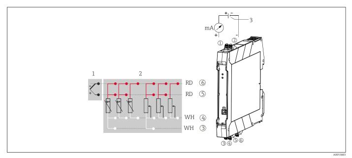
$\blacksquare 10$  Assignment of terminal connections for DIN rail transmitter
