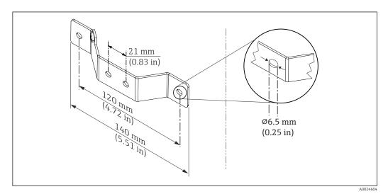
$\blacksquare$  4 Dimensions of angle bracket for wall mount (complete wall mounting set available as accessory)
