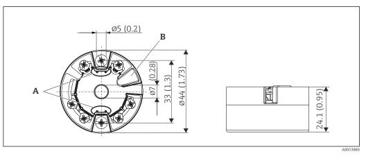
$\blacksquare$  19 Head transmitter version with screw terminals. Dimensions in mm (in)
