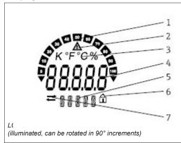
Item 1: Bar graph display in 10% increments with indicators for overranging / underranging
